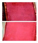
Above: This is the control sample, cast without metakaolin. There isn't much color difference compared to the samples with metakaolin, but there is a slight color shift. Below: In this sample we replaced 20% of the portland cement with metakaolin. When we diamond polished a portion of it, there was a very noticeable difference in hardness compared to the control sample.Joe NasvikHow and where to use it
