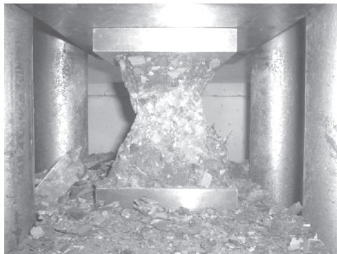
Figure 1--Concrete specimen after failure under compression.
