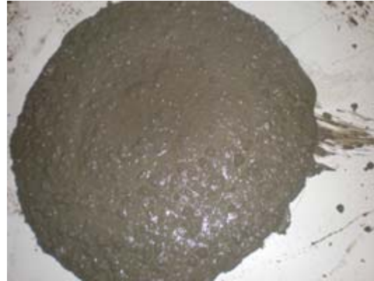
Self-consolidating concrete using metakaolin
